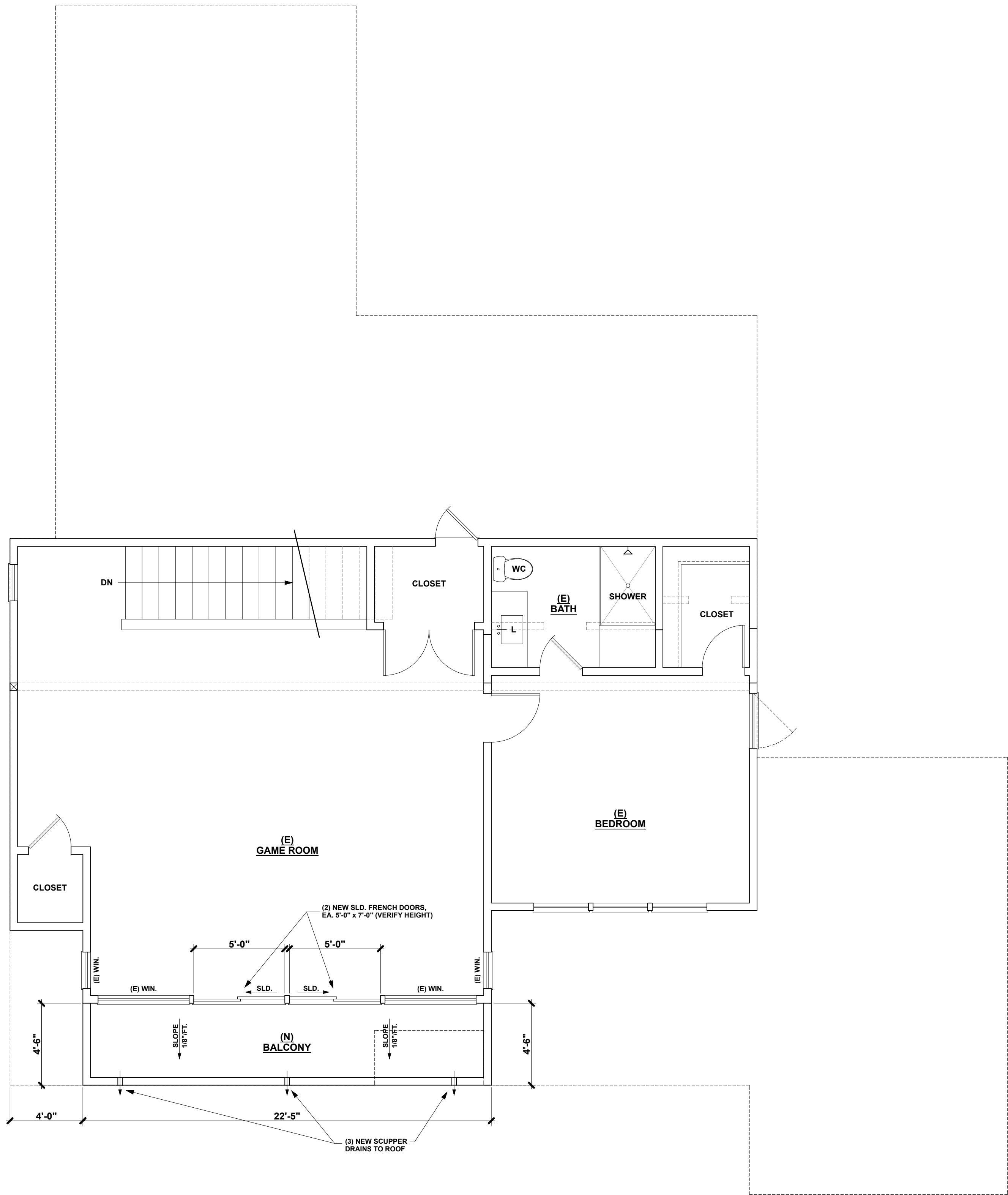
NEW BALCONY FLOOR PLAN (UPPER LEVEL) 1/4" = 1'-0"
