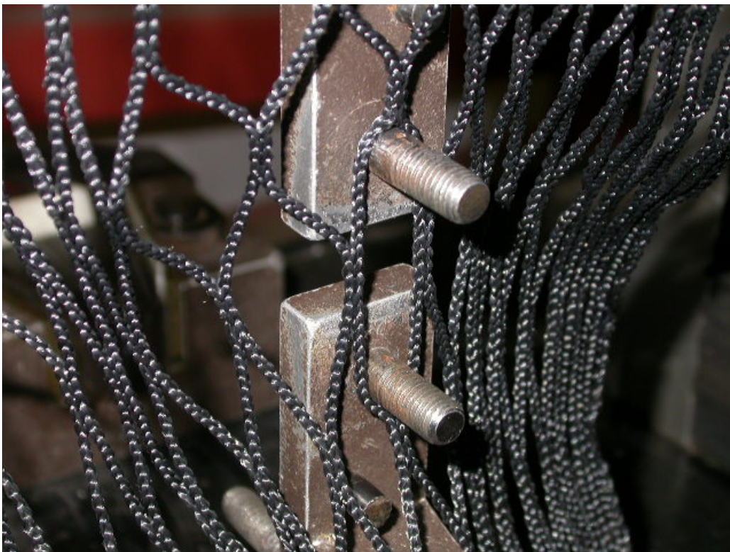
Figure 2. Break load testing in progress.
