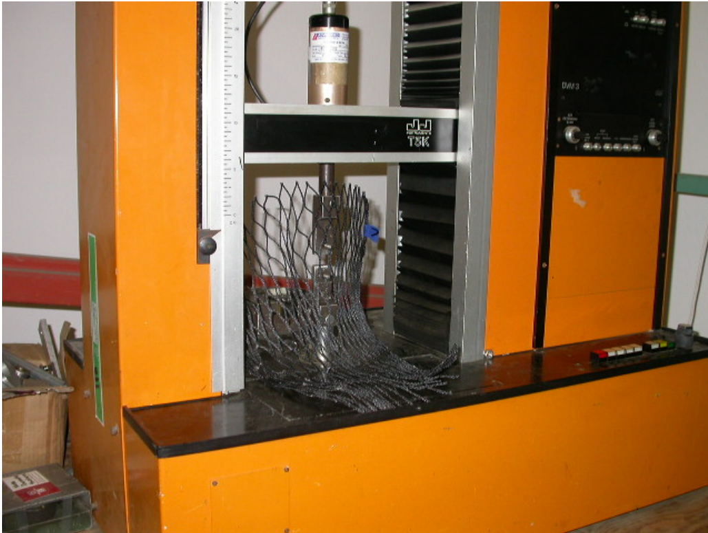
Figure 1. Tensile testing machine with net mesh in place for testing.
